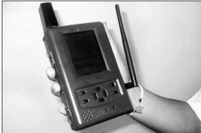
A handheld tactical computer developed for the Army.
